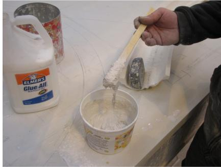
**9.** Use a sponge to wet the joint between the two light coves on back side (as shown below) and apply a 1/8" to a 1/4" layer of glassy mixture to backside of the joint. Apply some of the mixture 2" to each side of the joint (for additional strength). Use the sponge to smooth your mixture out. Let the mixture harden and then remove the clamp and/or shims.
