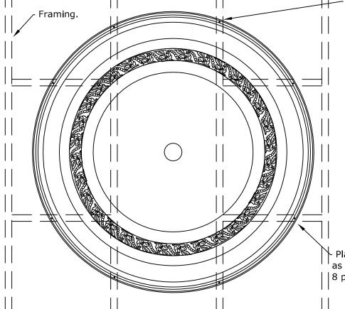
After you have marked all mounting points and a reference point to realign the dome to, predrill (1/8" bit) and countersink (1/4" bit), apply glue (construction adhesive) to flange, and mount to ceiling using 2-1/4" finish screws at all 8 framing points.
